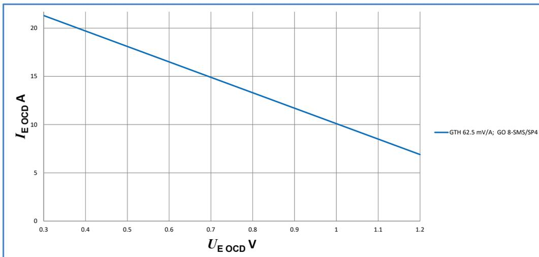
$$I_{E\text{OCD}} = \frac{(V_{ref} - U_{E\text{OCD}})}{G_{Th}} \times 1000 \quad U_{E\text{OCD}} = \frac{R_E}{R_E + R_{ref}} \times V_{ref}$$
